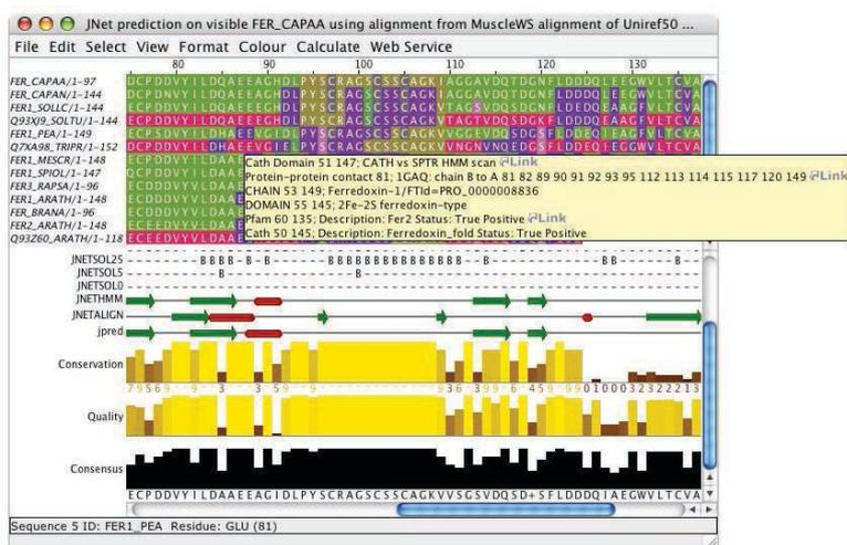
Figure 4.4: **Multiple sequence features.** An alignment with JPred secondary structure prediction annotation below it, and many sequence features overlaid onto the aligned sequences. The tooltip lists the features annotating the residue below the mouse-pointer.
