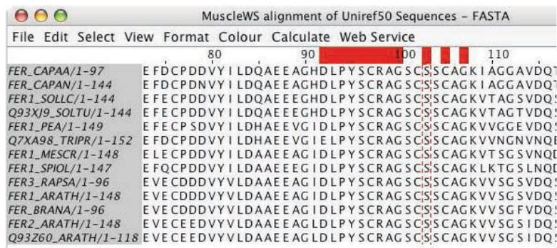
Figure 2.2: **Selecting multiple columns in an alignment.** The red highlighting on the alignment ruler marks the selected columns. Note that only the most recently selected column has a dashed-box around it to indicate a region selection.
